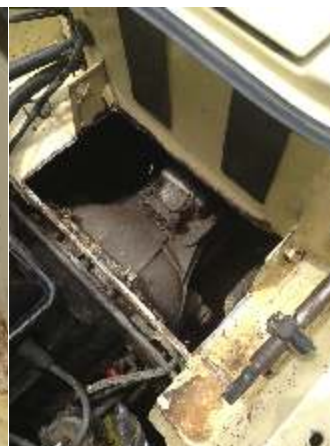
Rusted metal cut out.
